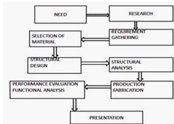
Fig. 1: Flow chart of design and fabrication methodology
